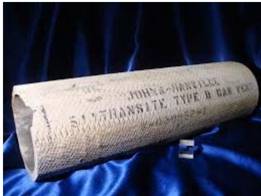
Example of transite duct.
